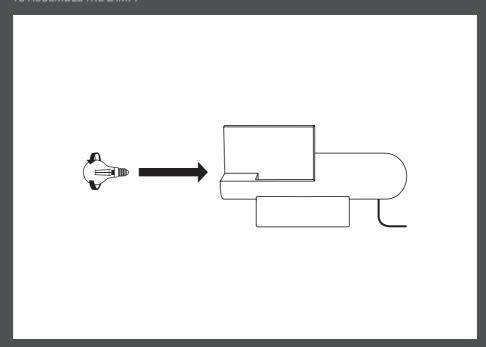
Place a recommended light bulb in the E14 socket. Light bulb is not included.
