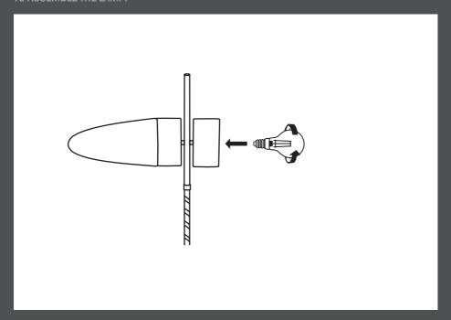
Before mounting the lamp shades, place a recommended light bulb in the E14 socket.
