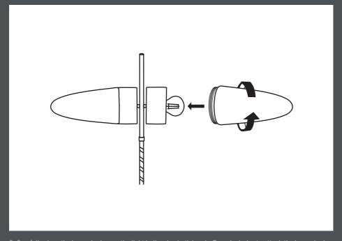
Carefully place the lamp shade over the light bulb using both hands. Turn clockwise to attach the lamp shade.
