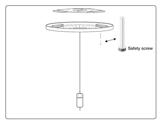
Remember to secure ceiling plate with safety screw to prevent detachment from ceiling plate.
