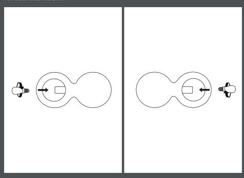
1. Place a recommended light bulb in the E14 socket.
