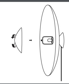
5. Install 185mm diameter lampshade. Turn clockwise to attach to the trestle.
