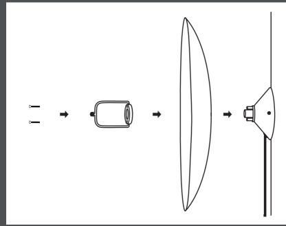
3. Attach the trestle and the 600mm diameter lampshade to the wall box using set screws.
