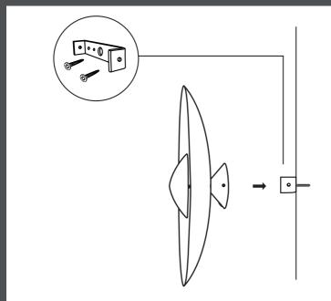
1. Detach the mounting plate from the wall lamp and mount it to the wall. Make sure to use appropiate screws and rawlplugs/anchors. Mount the wall lamp to the plate on the wall using the plated screws.
