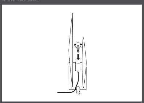
1. Place a recommended light bulb in the E14 socket. Light bulb is not included.
