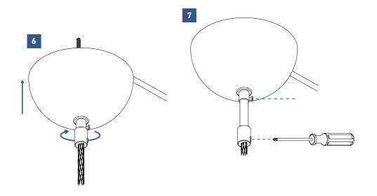
Lift the canopy so the thread sion tube is visible. Tighten the strain relief to the suspension tube.
