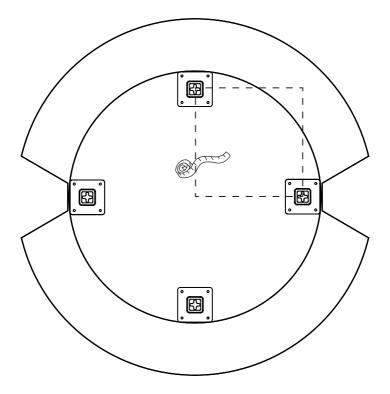
Use minimum 2 brackets for wall mounting. 3rd and 4th bracket is optional.
