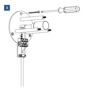
Remove the drill guide and fix the wall bracket to the wall, by using screws and rawplugs that match the wall type.
