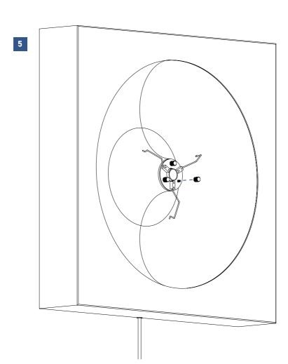
Place the globe fixture in the center and fasten it with the finger knobs.
