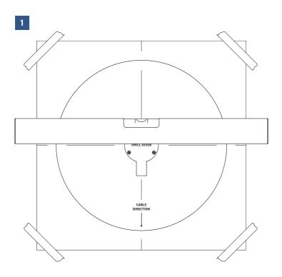
Place the drill guide on the wall and use a spirit level to level the horizontal line with the drawing. When in level, tape the guide to the wall.
