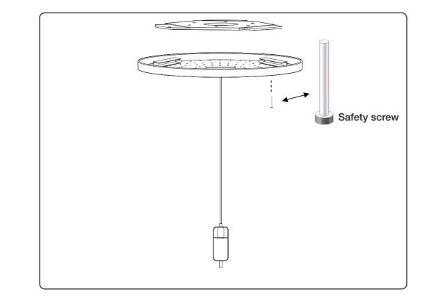
Remember to secure ceiling plate with safety screw to prevent detachment from ceiling plate.
