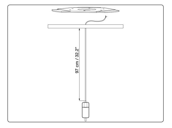
Pull the cord through the hole in the ceiling plate. The cord should measure about 97 cm - measured from the plate to the socket.
