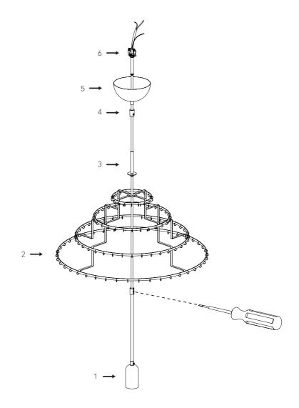
The wire must be secured. Read step 3. Important! that the weight of the lamp, is entirly in the wire.
