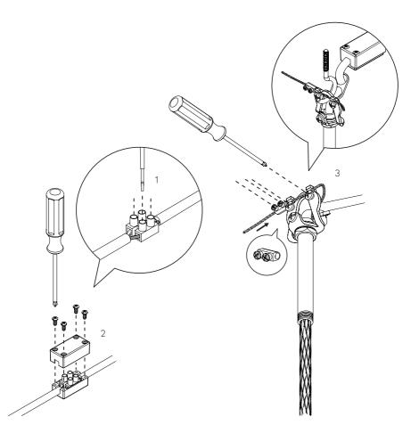
5 Lift the canopy so the thread at the bottom of the suspension tube is visible. Tighten the strain relief to the suspension tube.
