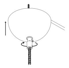
6 Lift the canopy to the ceiling and tighten the screw on the canopy. Tighten the set screw on the strain relief.
