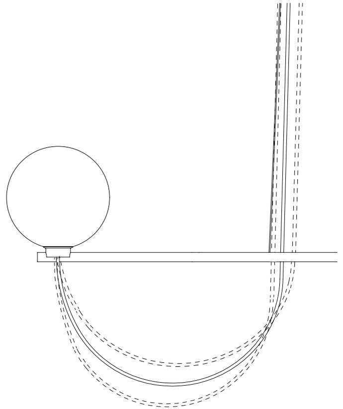
Unscrew the cable reliefs on the ceiling case. Pull the cable through to find the preferred length. Fabric Cable lengths: 5m. Ensure correct alignment. The cables should not cross over.
