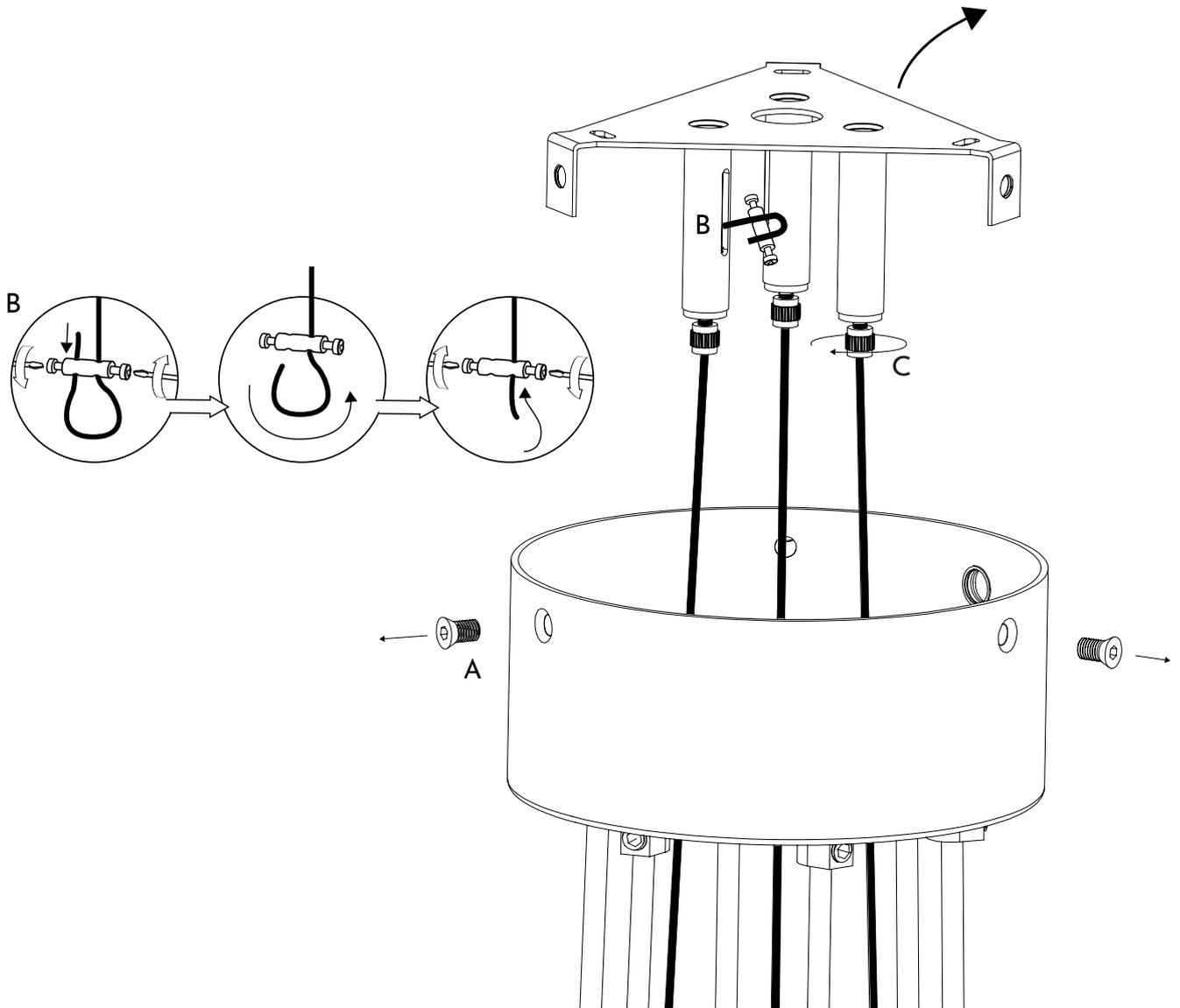
A - Unscrew the 3 x ceiling case screws so the bracket can be removed.
