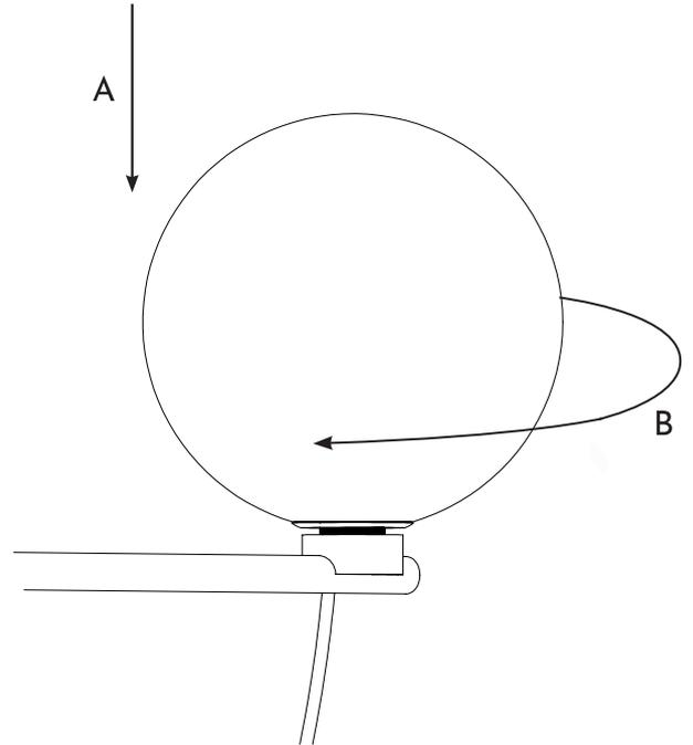
Take a glass globe and carefully place it over the light bulb and socket.
