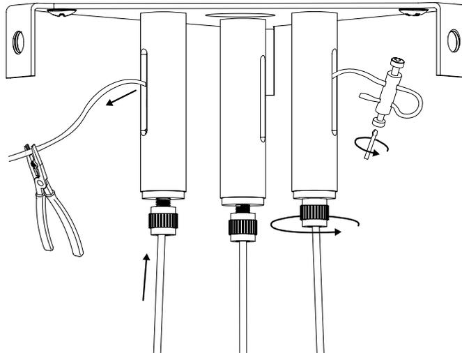
Align the wires from the frame with the wire locks. They must not twist.
