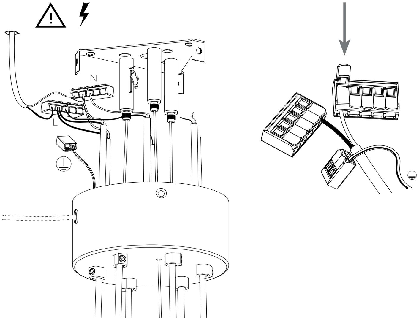
Check that the power is turned off before commencing any wiring. Lead all wires into the two connectors as shown. Ensure the wires are enclosed and secure when the orange lever is pulled back down.
