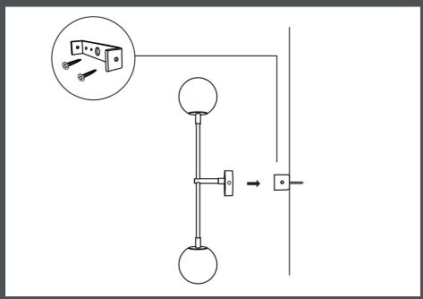
1. Detach the mounting plate from the wall lamp and mount it to the wall. Make sure to use appropriate screws and rawlplugs/anchors. Mount the wall lamp to the plate on the wall using the plated screws.
