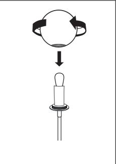
3. Place a recommended light bulb in the E14 socket
